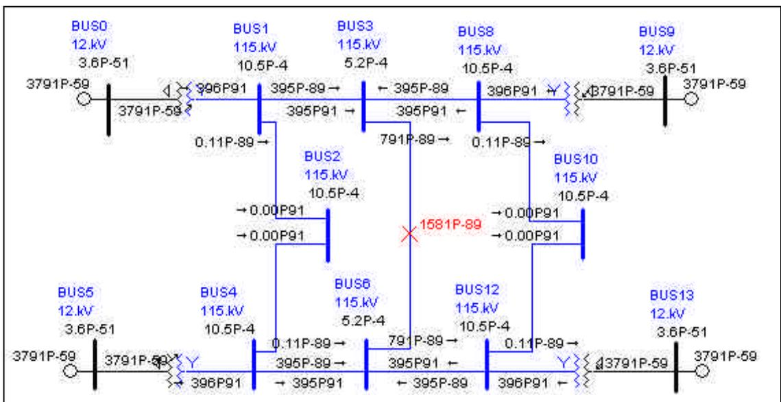
**Figure 3: Fictitious System Showing 3-phase Fault Values**
