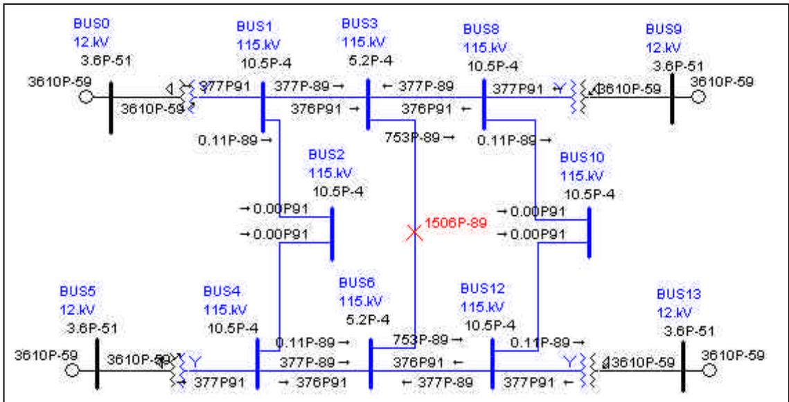
Figure 5: Fictitious System Showing 3-phase Fault Values
