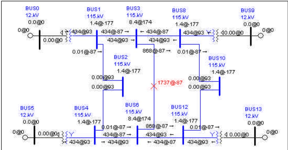
Figure 4: Fictitious System Showing Ground Fault Values
