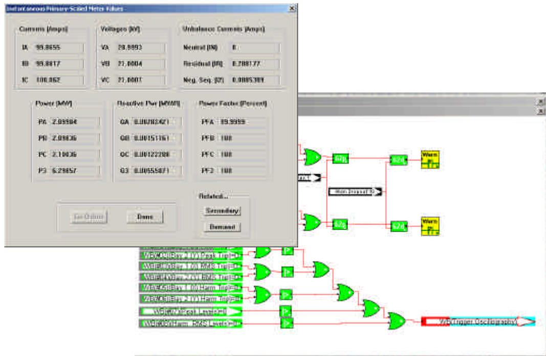
Figure 8: Example Manufacturer Monitoring Software Showing Logic States and Metering
