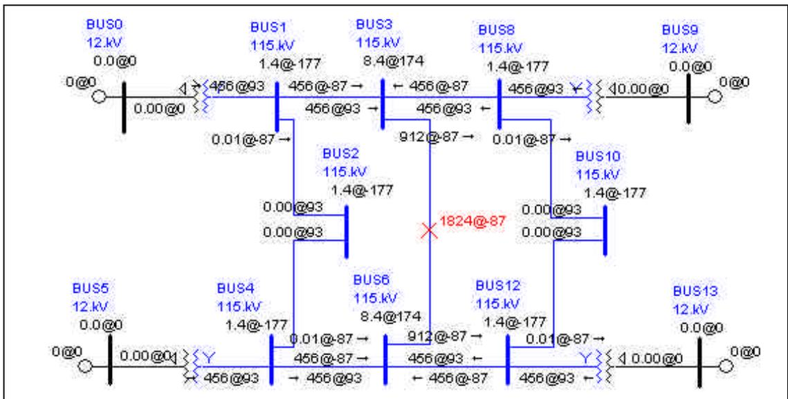
**Figure 2: Fictitious System Showing Ground Fault Values**
